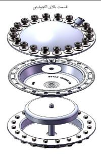
In some cases, the pressure is exerted inappropriately and in a pulsing way on the diaphragm. In that case, clean the lines and connections in order to avoid clogging. If the valve is installed in the opposite direction, it will result in a lower pressure than the set point. If there is pressure after the valve, the valve is too big and its size must be checked. If necessary, the smaller Kvs coefficient shall be selected.
